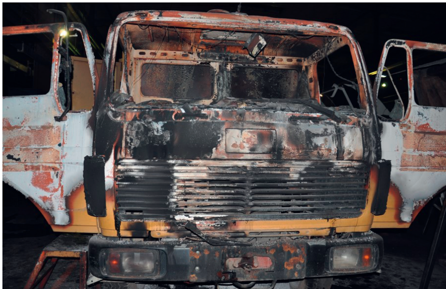
Photograph 6. The appearance of a truck in which fire started in the cabin due to a short circuit on the installation around the fuse
